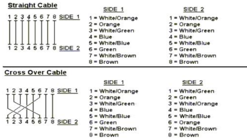
Figure A-1: Straight-Through and Crossover Cable
